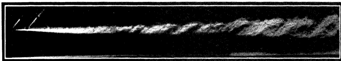
Fig. 5 Composite schlieren for M_c = 0.28 , x = 0-45 cm (flow is from left to right).
